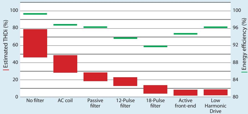
A comparison between different harmonic mitigation principles shows that low harmonic distortion is followed by low energy efficiency – except for active filtering, where the efficiency is relatively good.
